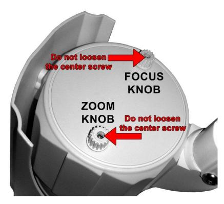
**NOTE:** The tension of these knobs is set at the factory for maximum weather protection. <u>Do not</u> <u>loosen the screws which hold the knobs in place</u>. This could cause the adjustment rod to fall inside the camera and will void the warranty. If the screws are difficult to turn by hand, pliers may be used.
