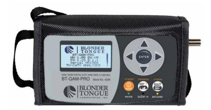
The BT-QAM-PRO is an economical feature packed test instrument for analyzing CATV QAM and Broadcast 8VSB digital channels, as well as NTSC analog channels. This compact instrument is designed with field service technicians in mind, and provides many of the features that are typically only found in much higher priced units. The BT-QAM-PRO comes complete with a soft water resistant case and a micro USB charging/PC cable.
